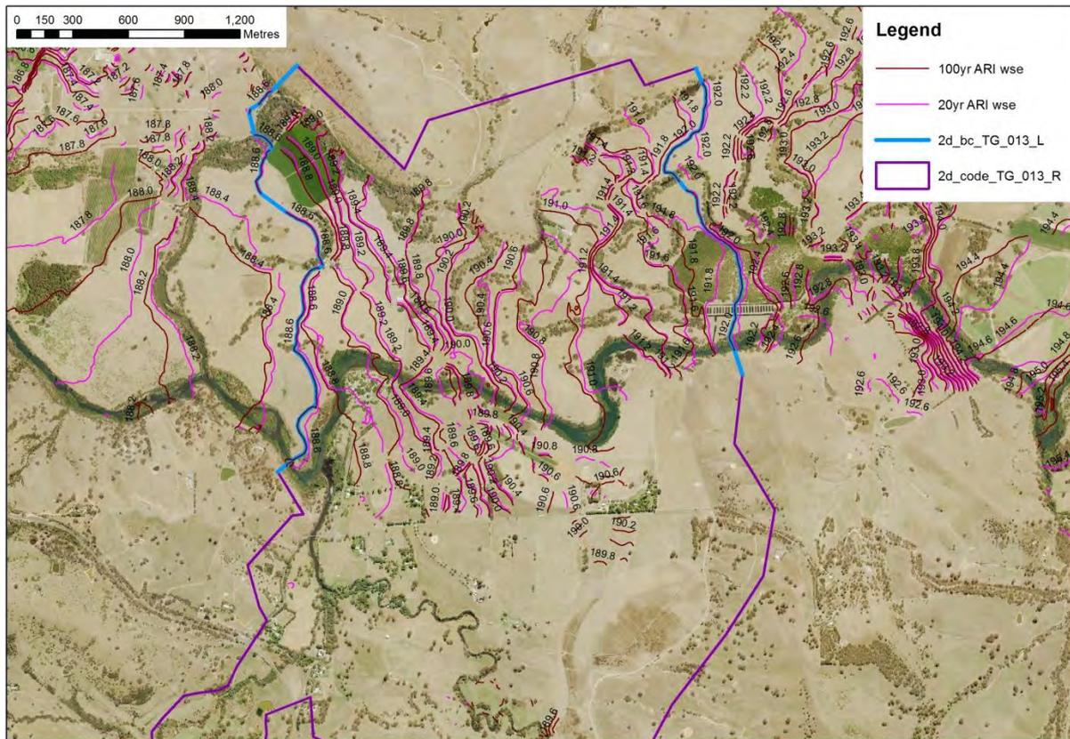
**Figure 4-1** The confluence of the Acheron and Goulburn Valleys showing the Constraints Project 20 year and 100 year ARI water level contours and locations of inflow (right, u/s) and outflow (left, d/s) boundaries for the Acheron hydraulic model.
