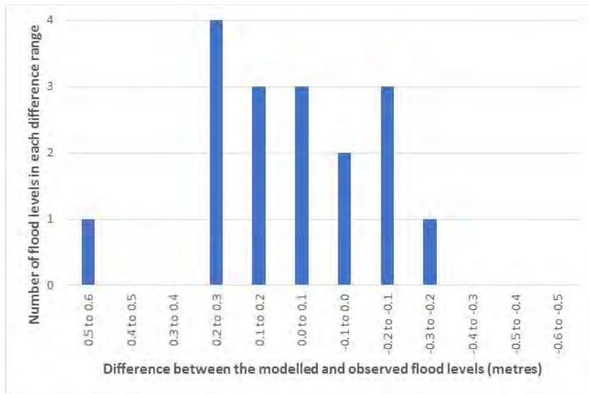
**Figure 5-3** The number of flood levels in each range of difference for the 1996 flood at Buxton. The difference is the modelled flood level minus the surveyed (observed) flood level.
