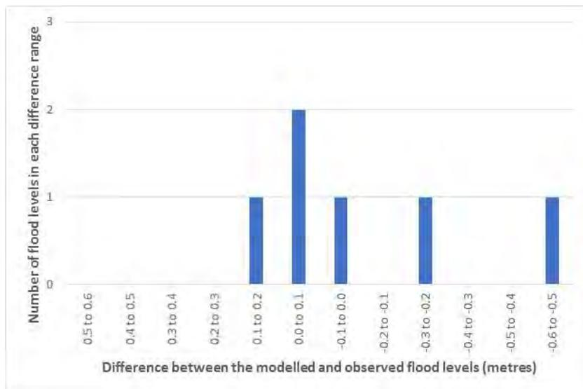
**Figure 5-7 The number of flood levels in each range of difference for the 2010 flood at Taggerty.**
