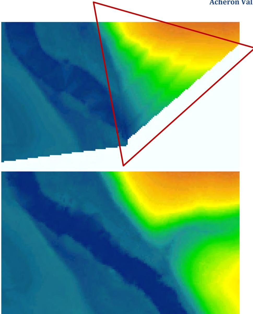
**Figure 3-5** North East Towns LiDAR (top) and ISC LiDAR (below) on the Acheron River at E385640 N5865980. The red triangle shows the extent of the distorted LiDAR.
