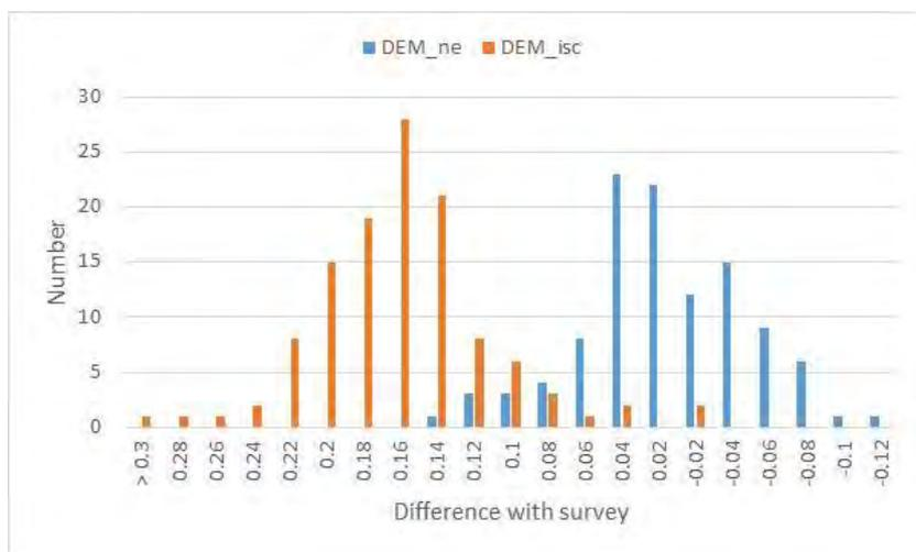
**Figure 3-4** Histogram of the difference between survey levels and DEMs at Taggerty.
