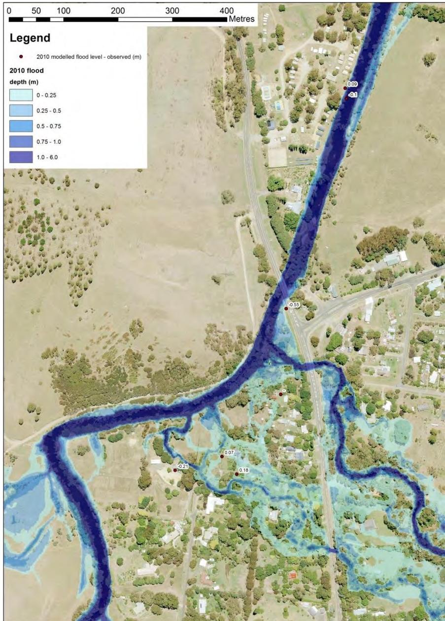
**Figure 5-8** The modelled flood extent and depths for the 2010 event at Taggerty. Modelled flood levels minus the surveyed (observed) levels are also shown.
