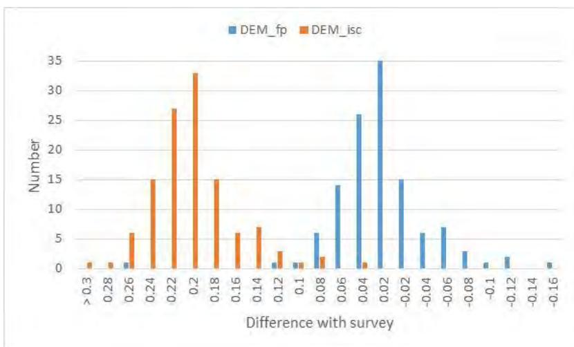
Figure 3-2 Histogram of the difference between survey levels and DEMs at Buxton.
