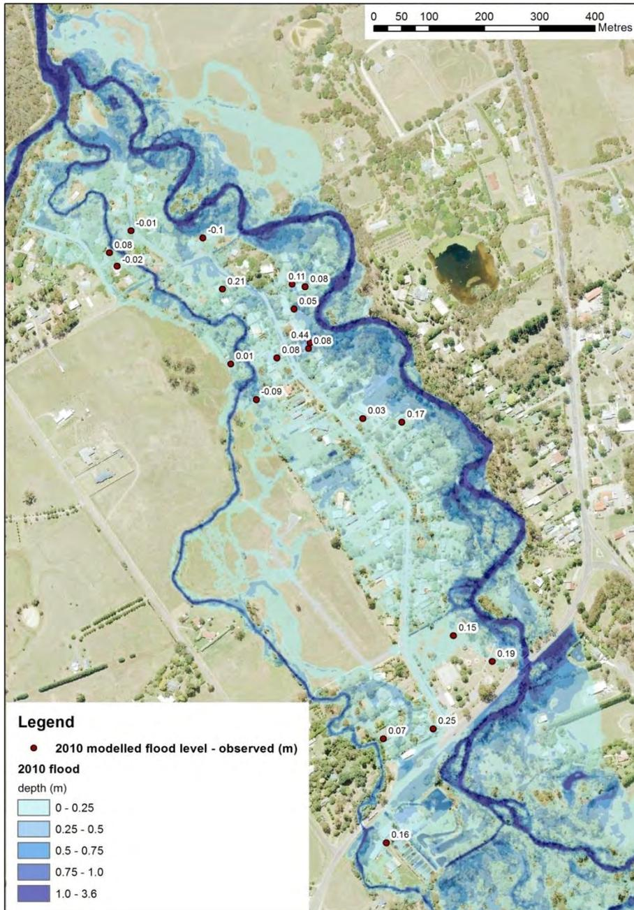
**Figure 5-5** The modelled flood extent and depths for the 2010 event at Buxton. Modelled flood levels minus the surveyed (observed) levels are also shown.
