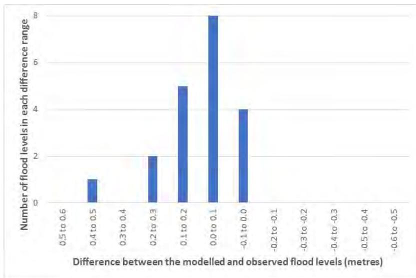
**Figure 5-4** The number of flood levels in each range of difference for the 2010 flood at Buxton.
