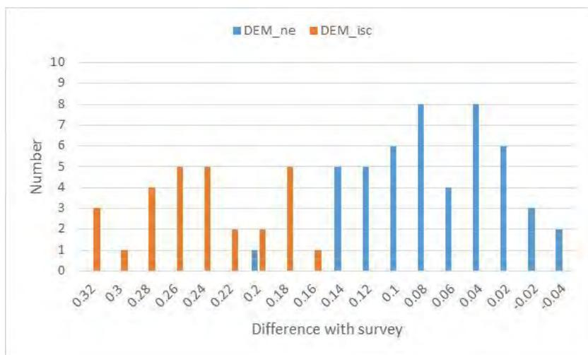
**Figure 3-7** Histogram of the difference between survey levels and DEMs at Marysville.
